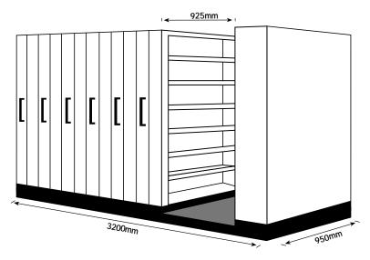
This illustrated example represents a typical Video Maxtor installation, featuring six doubleface Video storage bays, with a 300mm deep plinth (fixed bay) for larger items. This configuration, with 2000mm high x 900mm wide bays, would have the capacity to store up to 2436 VHS video cassettes (30mm wide).
